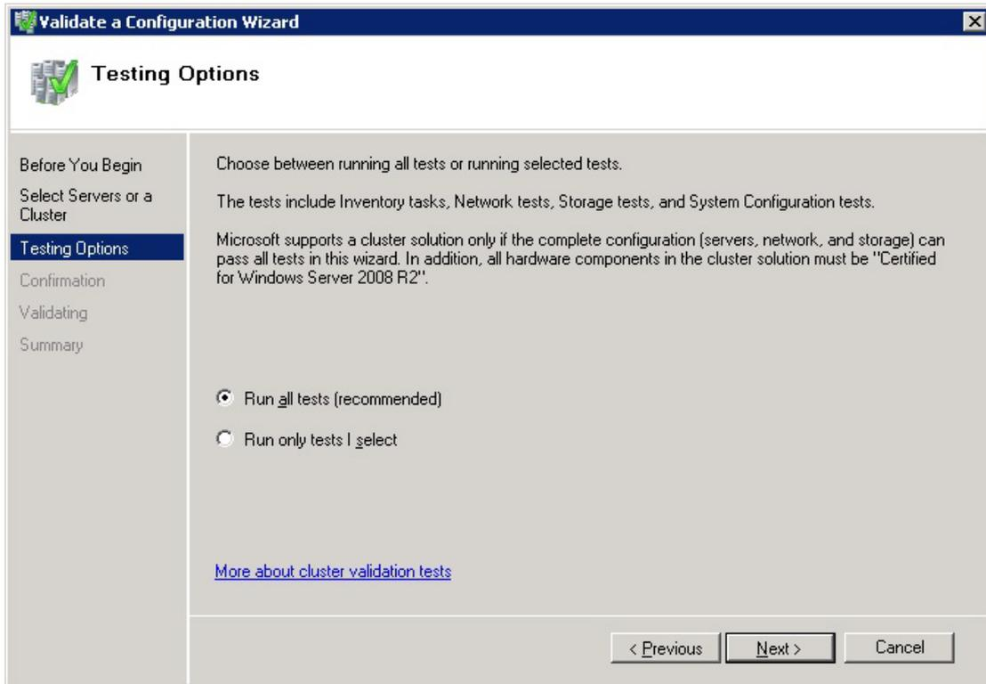
Select **Run all tests (recommended)** and Press the **Next** button to continue.
