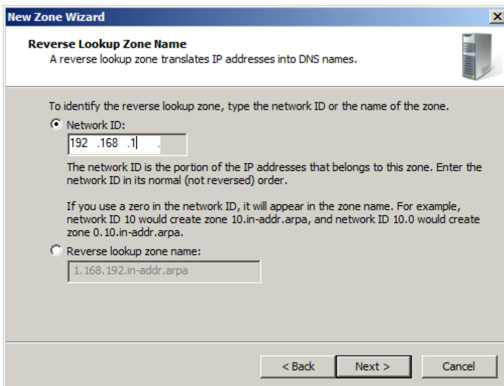
Select the **Network ID** and then type the IP address in the **Network ID**
