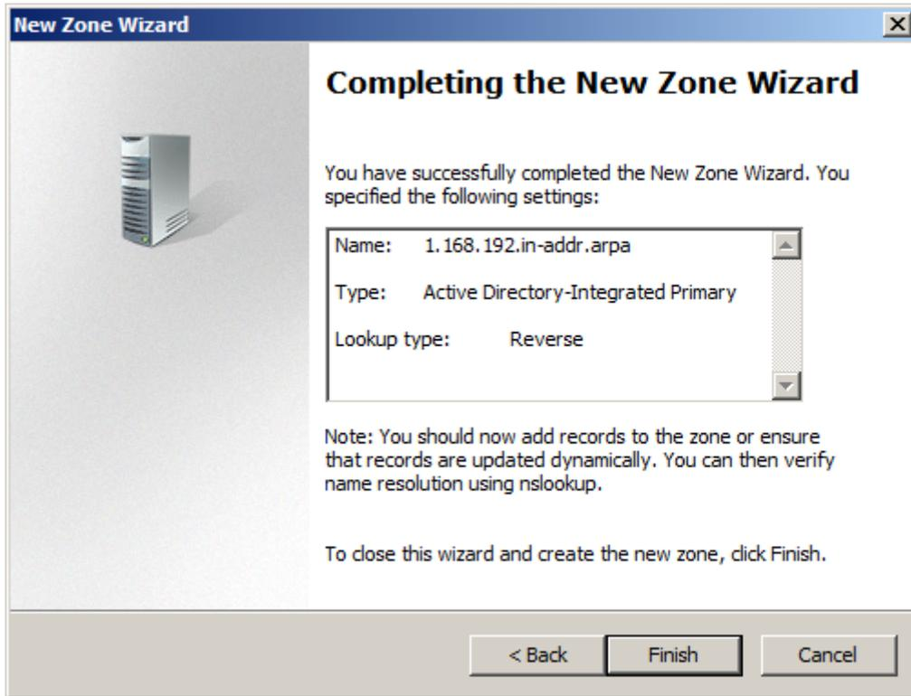
Check all of the parameters are correct, and press **Finish** to create the new zone.
