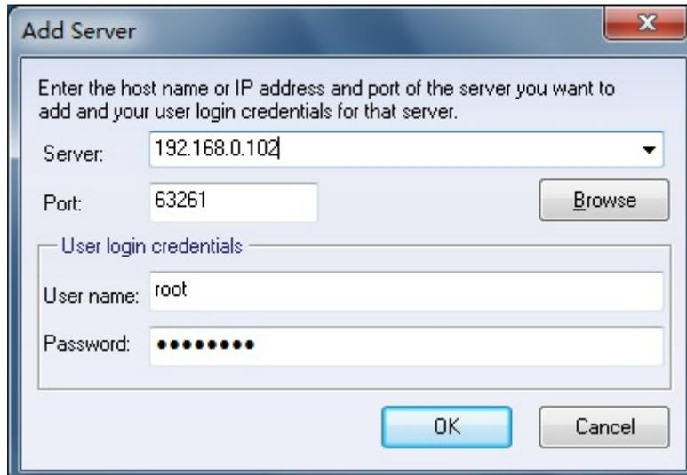
After pressing **OK** button to save setting and connect to the server, HAReplicator Management Console will be shown as below
