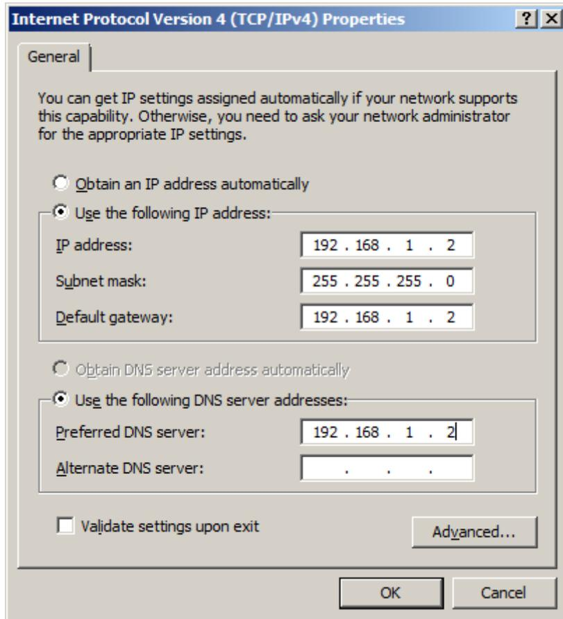
Fill in the IP address and the DNS server must point at itself address.
