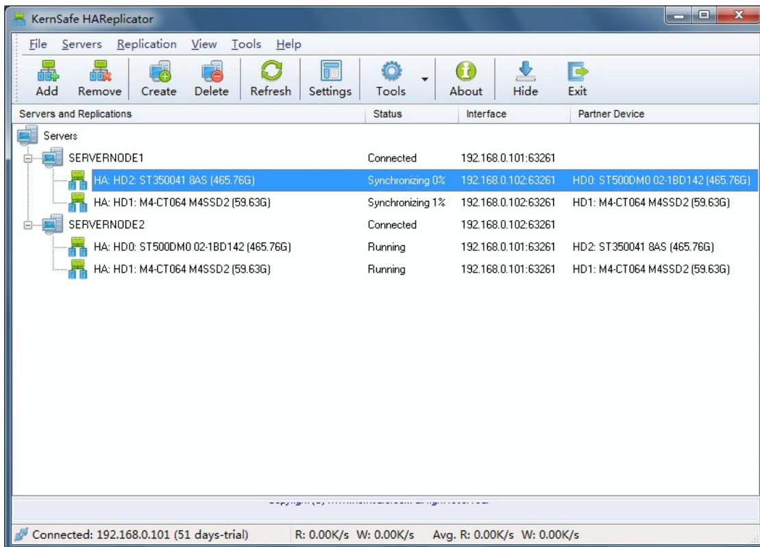
After synchronization completes, you can put the disks into MSCS.
