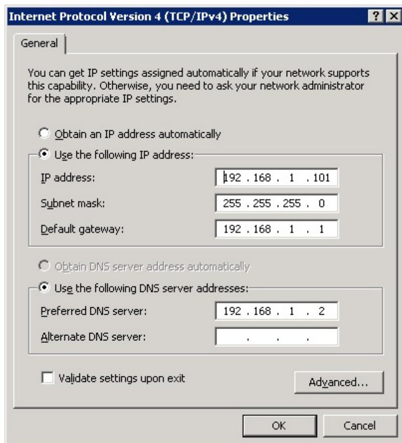
Type the **IP address** , **Subnet mask**, **Gateway** and **DNS server** .
