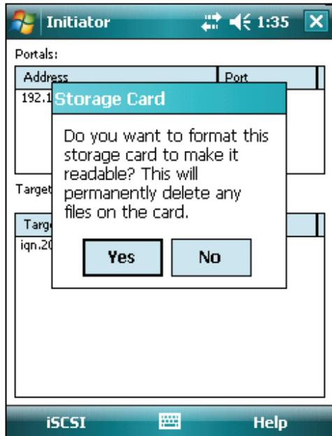
This is because we connected to RAW target that was created in iStorage Server. This information will appear only for the first time using this target.
