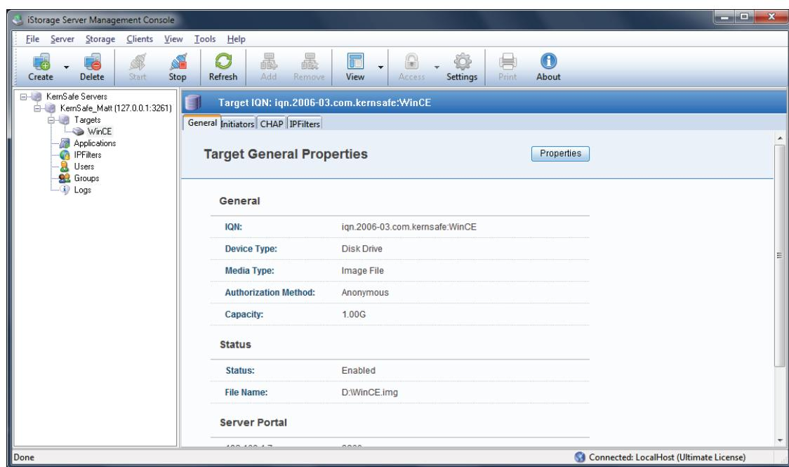
We successfully created iSCSI Target. We can now connect to it using KernSafe WinCE iSCSI Initiator.
