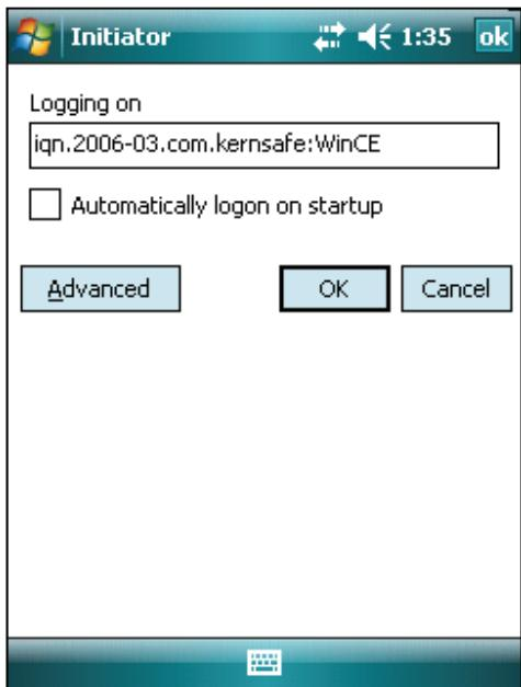
Checking **Automatically logon on startup** option will result that target will be automatically mounted upon turning on the device.
