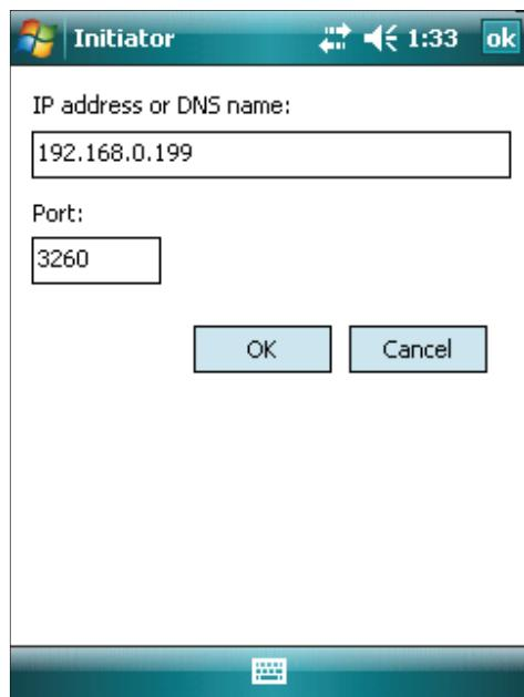
After finishing, tap on **OK** button to connect to the portal. You will notice that portal was successfully discovered as well as all targets within this portal.
